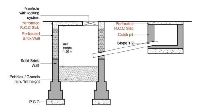
**b. For Buildings with building-unitarea above 500sq.mt and up to 1500 sq.mt:** Percolating Well with Rainwater Harvesting System shall be provided as illustrated below (up to ground first river):
